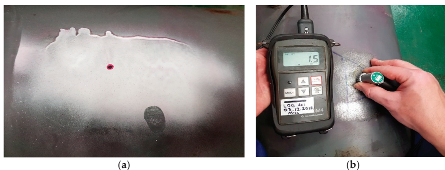
Figure 2. Example of non-destructive testing of rotating machinery equipment: (a) liquid penetrant testing, (b) ultrasonic thickness testing.
