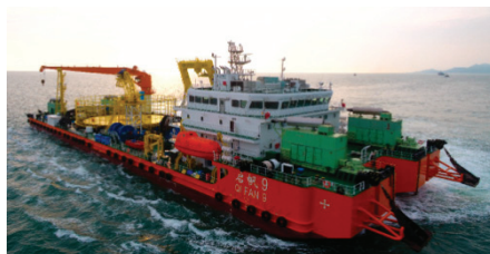
Figure 1. Qifan No. 9 with a cable capacity of 5000 tons.
