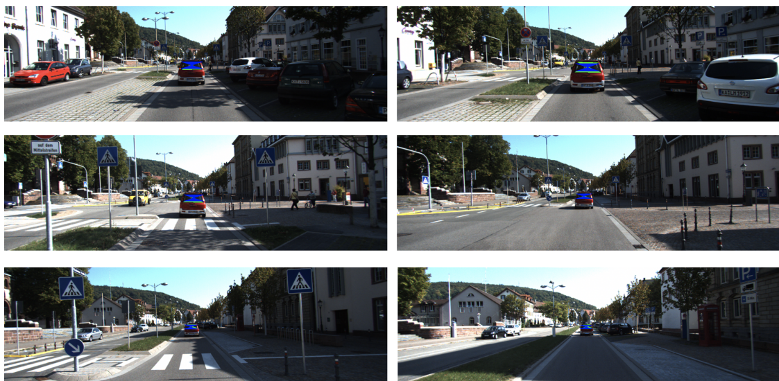
Figure 3. The results of the algorithm pipeline focusing on an ego lane car. The estimated 3D position of the rear windshield corners (in blue) are superimposed on the image against the ground truth position (in green).
