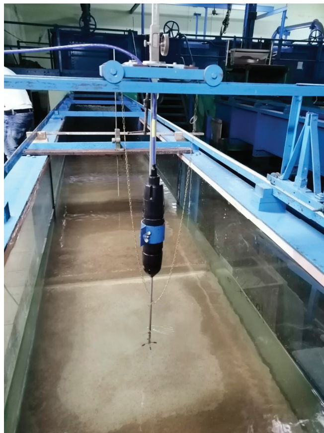
Figure 2. The flume setup for the sand-bed (Run 1 and Run 2).
