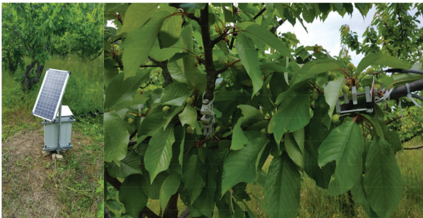
Figure 1. Acquisition system, with a CR100X datalogger (Campbell Scientific Inc., Logan, UT, USA) and an automatic extensometer DEX20 (Dynamax Inc., Huston, TX, USA).
