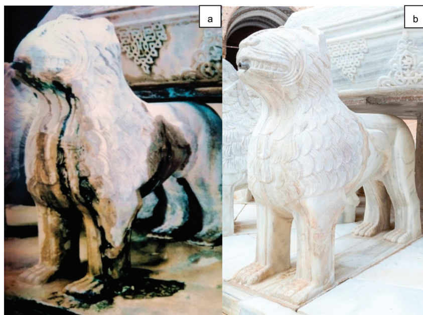
Figure 10. Presence of microalgae on one of the lions in the Fountain of the Lions: (a) an image from 1994 by F. Bolivar is shown on the left; (b) a modern image by G. Alfano in which one can see the effect of the cleaning treatment and lack of large sheens on the surface is shown on the right.
