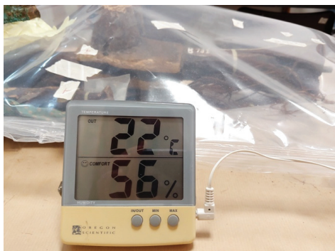
Figure 7. “Clean chamber” assembled for exposure (7 weeks) of the wooden sculpture to T. vulgaris EO volatile compounds. Inside/outside temperature ( 22 \pm 1 °C) and relative humidity ( 56 \pm 2\% ) values were continuously monitored by an Oregon thermo-hygrometer equipped with a microprobe.
