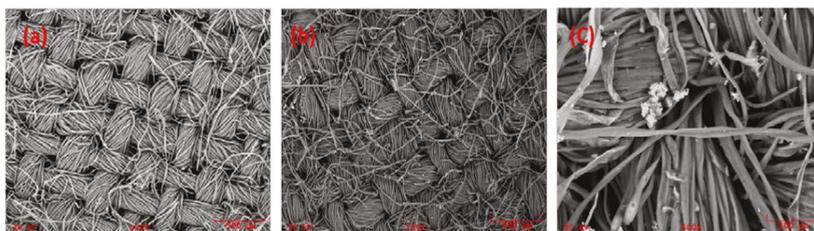
**Figure 3.** Scanning electron microscopy images of (a) uncoated cotton (100%) cellulose fabric substrate at 100 $\times$  magnification; (b) uniformly coated sol–gel C18 sorbent coating on fabric matrix at 100 $\times$  magnification; (c) sol–gel C18 coated FPSE media at 500 $\times$  magnification.
