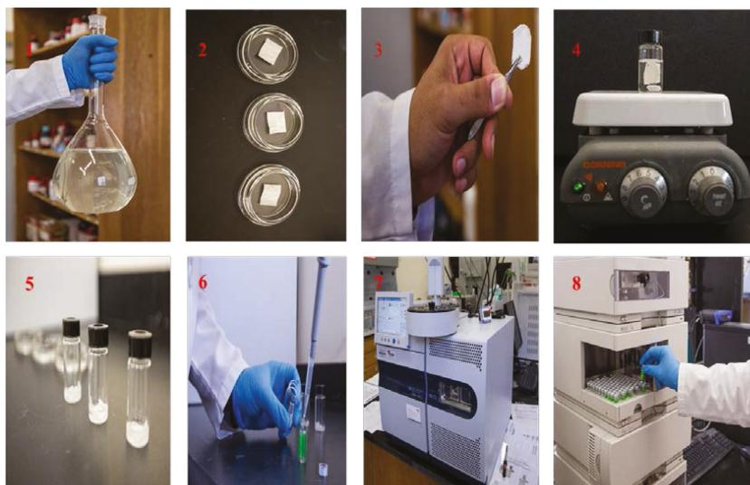
**Figure 1.** Steps in fabric phase sorptive extraction (FPSE): (1) unfiltered, dirty environmental sample; (2) FPSE media on watch glass; (3) an FPSE medium on a tweezer; (4) fabric phase sorptive extraction; (5) back-extraction in organic solvent; (6) transferring preconcentrated eluent into sample vial; (7) analysis in GC; (8) analysis in HPLC.
