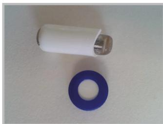
**Figure 2.** Magnetic molecularly imprinted stir bar (MMISB) developed for the extraction of patulin; a screw cap was placed below the stir-bar to illustrate its size (Reproduced with permission from [11]. MDPI under [CC BY 4.0](https://creativecommons.org/licenses/by/4.0/), 2015).
