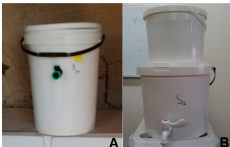
Figure 2. The Household water treatment systems (HWTS) implemented in Makwane Village; (A) BSZ-SICG filter and (B) SIPP filter.
