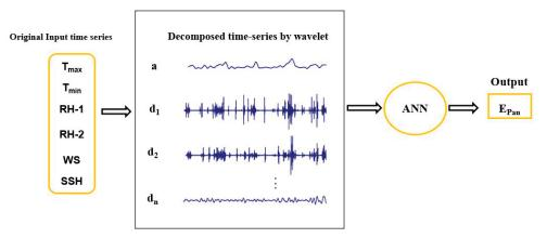
Figure 4. Schematic representation of WANN.
