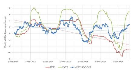
**Figure 2.** Comparison of the in situ vertical displacement of both extensometers (EXT1 and EXT2) to VERT-ASC-DES, the vertical displacement using the ascending and the descending track of Sentinel-1 at West Point (WP). The linear trendlines of the displacements are also shown (dotted lines).
