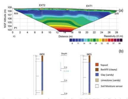
**Figure 3.** (a) Vertical cross section of resistivity along P1 profile (EXT1-EXT2). (b) Clay depth and thickness at EXT1 and EXT2 deduced from the resistivity profile (see text). E1 sensor (near EXT1, Figure 1) and W5 (near EXT2) are both located at the same 1.2 m depth inside the clay layer.
