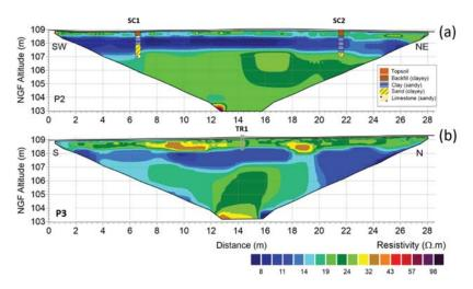
**Figure 4.** (a) Vertical cross section of resistivity along P2 profile (SC1-SC2) showing the SC1 and SC2 geological logs. (b) Vertical cross section of resistivity along P3 profile (South-North) showing TR1 drilling.
