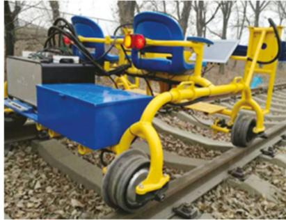
**Figure 7.** Intelligent track inspection vehicle.
