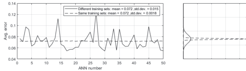
Figure 5. Neural network error dispersion comparison between using same versus different training data.
