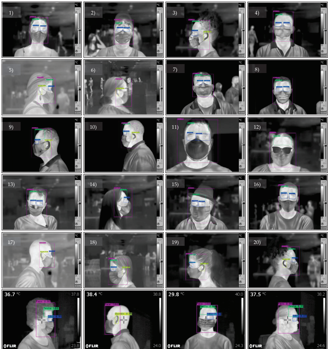
Figure 12. Images produced using the Testo-885 camera and analyzed by YOLO, with temperature estimated using Equation (3).
