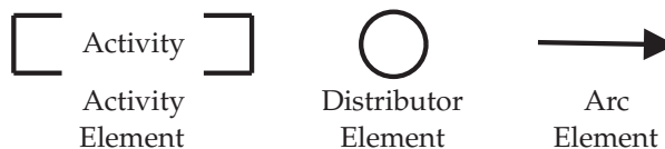
Figure 1. Basic elements of the Production Flow Schema (PFS). The PFS represents the system conceptual description. Arcs connect activity and distributor elements. Activity elements can be refined into a new PFS model or a PN.
