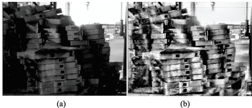
Figure 4. Enhancing image features: (a) original image and (b) adaptive histogram equalization.
