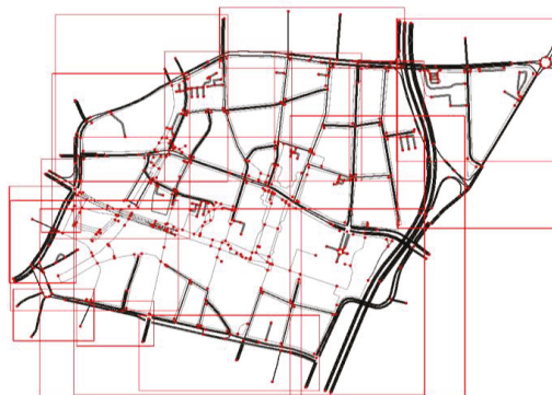
Figure 4. Traffic Assignment Zone (TAZ) distribution of Duisburg inner ring; each red box shows the roads in one TAZ.
