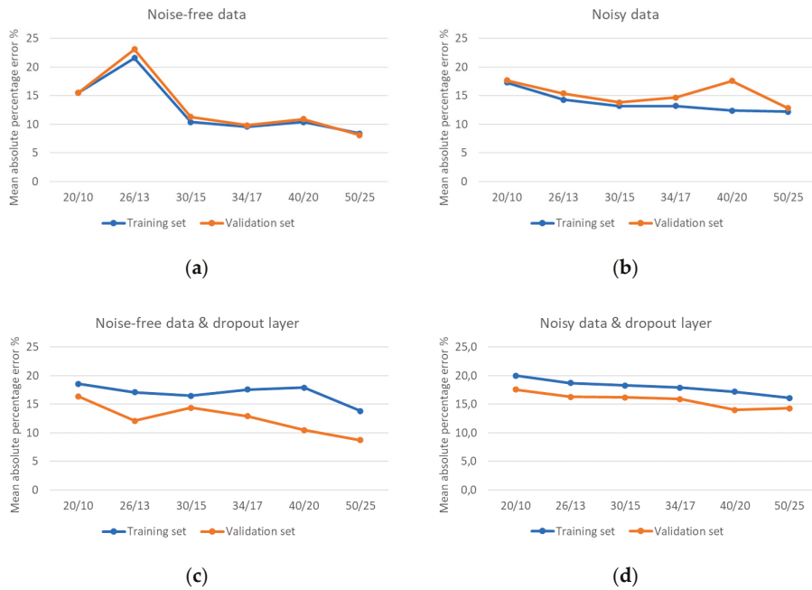
Figure 8. (a–d): Mean absolute percentage error obtained for various network architectures and with respect to existence of noise in the training and validation data sets.
