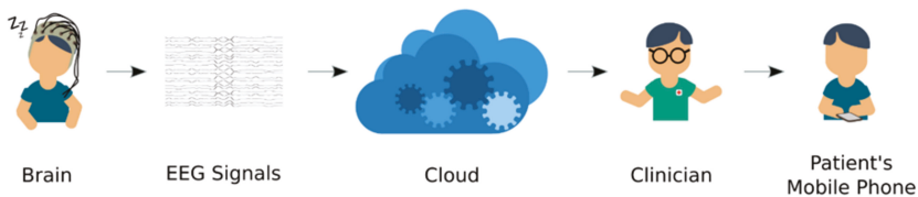
Figure 15. Block diagram of cloud-based sleep stage classification system using EEG signals.
