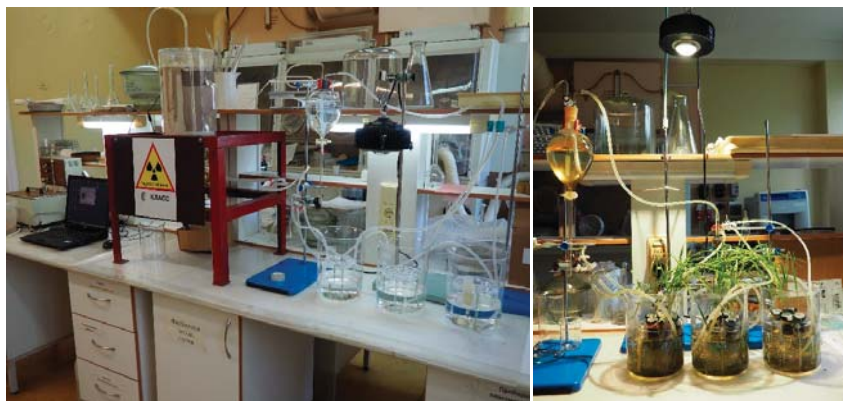
Figure A1. A stand for studying the parameters of ^{65}\text{Zn} (Zn) migration in the soil–soil solution–plant system: 1—the moment of equilibration of deionized water in the system with Albic Retisol (Loamic, Ochric) soil; 2—vegetative vessels with plants.
