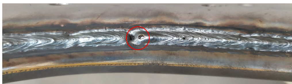
Figure 10. Defects when using incorrect welding parameters ( I = 210 A, v = 80 cm·min -1 ).
