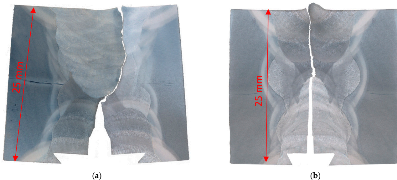
Figure 12. Crack path after fracture toughness testing of both specimens, etched by 4% Nital: (a) UM/OM configuration 1 (initial crack in UM); (b) OM/UM configuration 2 (initial crack in OM).
