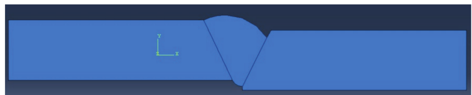
Figure 4. Model with vertical misalignment, incomplete root penetration, and undercut.
