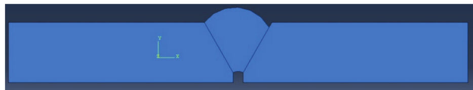
Figure 2. Model with excess weld metal, incomplete root penetration, and undercut.
