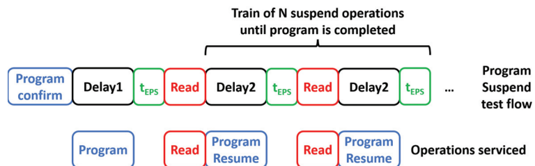
Figure 5. The program suspend test flow exploited in this work to explore the operation characteristics.
