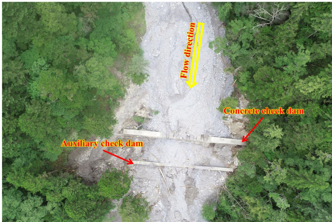
Figure 5. Overview of the reconstructed check dams in Zechawa Gully (taken on 25 June 2019).
