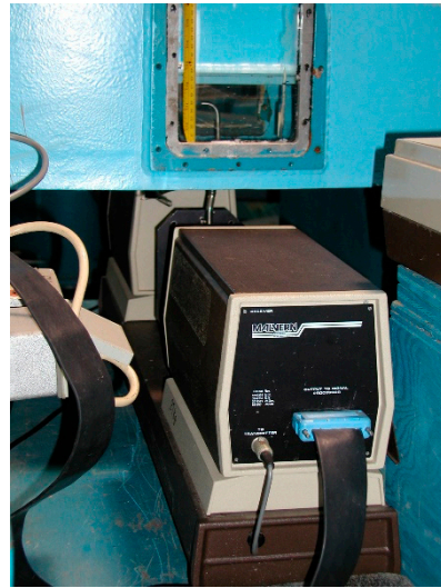
Figure 6. A photograph showing the placement of the Malvern instrument underneath the flume.
