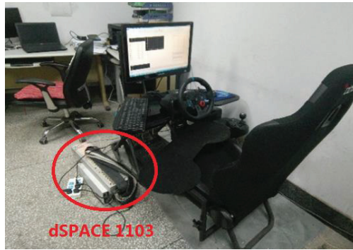
Figure 13. Testing simulator platform based on dSPACE hardware.
