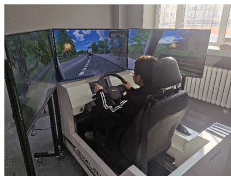
Figure 12. Driver-in-the-loop experiment to collect drivers’ reactions to different working conditions.
