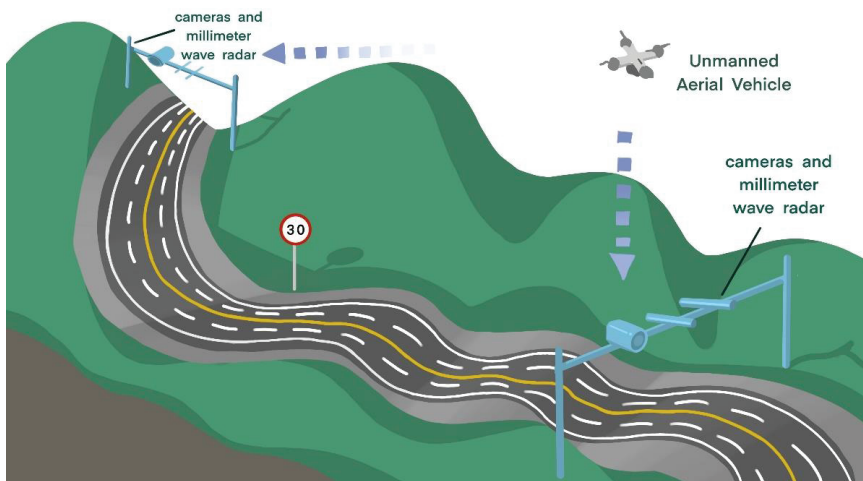
Figure 8. Use traffic sensors to collect changes in traffic parameters.
