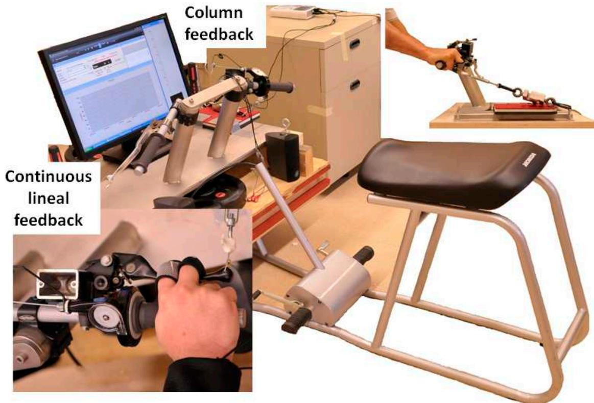
**Figure 2.** Simulation of the overall position of a rider above a motorcycle race from 600 cc to 1000 cc. A static structure was built to preserve the distances between seat, stirrups, and particularly the combined system of shanks, forks, handlebar, brake and clutch levers, and gas.
