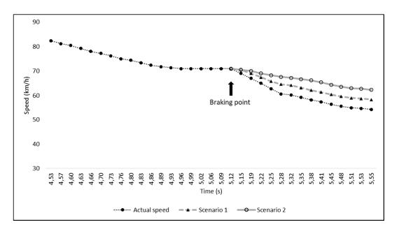
**Figure 9.** Rossi's actual speed (moving an average of 5 points), 33 frames before the point where he narrowly missed colliding with Morbidelli's careening bike. As described in the legend, the solid dots represent Rossi's real speed and the solid triangles represent the speed in hypothetical scenario 1, while the empty dots represent the speed in scenario 2.
