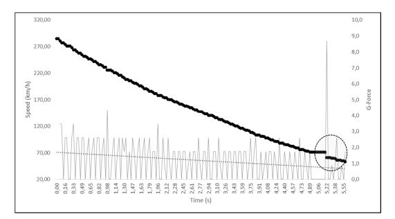
**Figure 8.** Rossi's actual speed and instantaneous G-Force peak from point A to the point where he narrowly missed colliding with Morbidelli's bike. The circled area shows the moment in which Rossi braked, reducing his speed by 10 km/h in 0.03 s.
