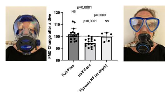
**Figure 2.** Flow mediated dilation (FMD) changes after a dive (10 m for 20 min) either wearing a full-face mask or a classical "half-face" diving mask (n = 16). In hypoxic dives (n = 5), subjects were breathing a gas mixture providing 0.16 ATA of PO<sub>2</sub> at depth. FMD changes are expressed as % of predive values, every diver acting as his own control. Results are expressed as percentage (mean  $\pm$  SD); NS = nonsignificant.
