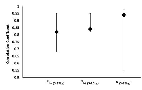
**Figure 2.** Median correlation coefficients and their ranges obtained comparing the vertical thrust's height free load with individual  $F_{bk}$ ,  $P_{bk}$  and v at 5–25 kg.
