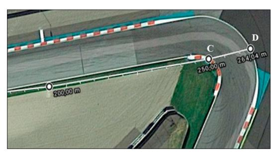
**Figure 5.** Satellite image showing the section of the straightaway leading into turn 3. Point C corresponds to a marker on the internal curb of turn 3, the point where Morbidelli's bike began cartwheeling across the track. Point D is shown by a marker on the outer edge of turn 3 with a trajectory that follows the line of the straightaway, the same trajectory that Morbidelli's bike followed as it cartwheeled across the curve. The line from C to D measures 14 m.
