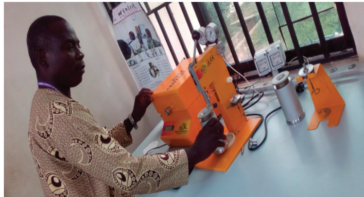
Figure 1. e-2k Combustion for HHV determination [27].
