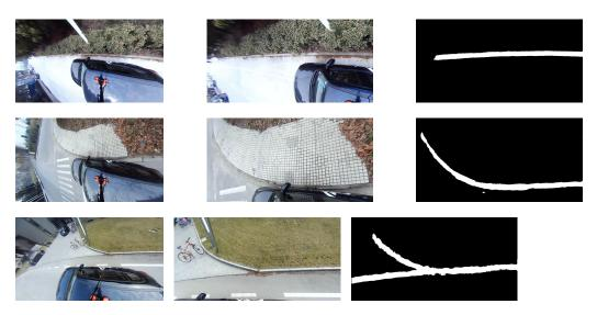
**Figure 3.** Detection results of deep curb detection network. Left column: image samples from the dataset; Middle Column: enlarged curb regions of interests extracted by CRoI module; Right column: curb segmentation results.
