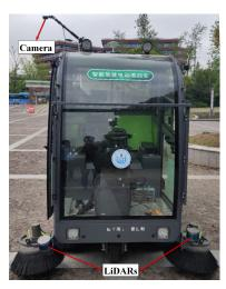
Figure 4. The intelligent sweeper of Tongji University.
