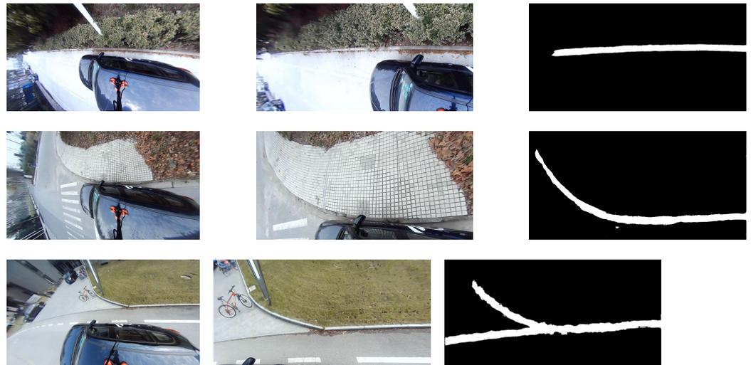
**Figure 3.** Detection results of deep curb detection network. Left column: image samples from the dataset; Middle Column: enlarged curb regions of interests extracted by CRoI module; Right column: curb segmentation results.
