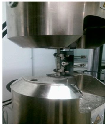
Figure 4. Tension specimen on the grips.
