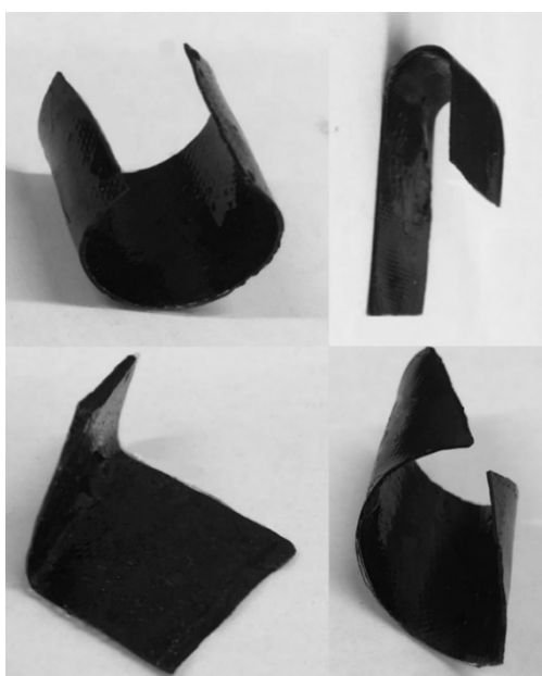
Figure 6. Different shapes of the MWCNT nanopaper/epoxy composites manipulated by hand after composite Joule heating to 70 °C and cooling below the T_g temperature of 53.9 °C to form new shapes.
