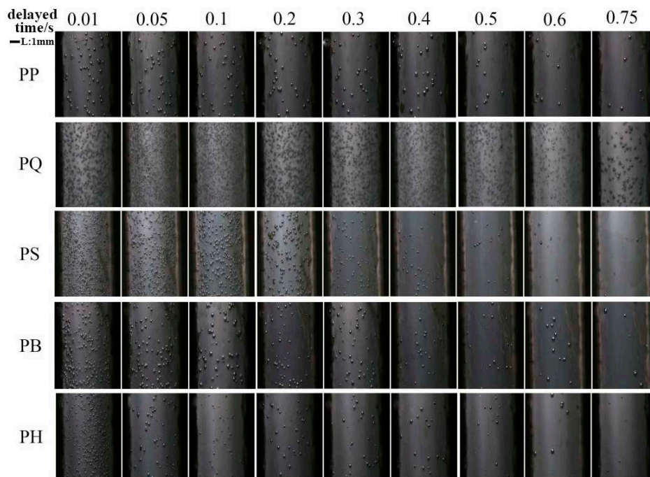
Figure 14. Pictures of the bubbles of the PP composite with different mold opening times.
