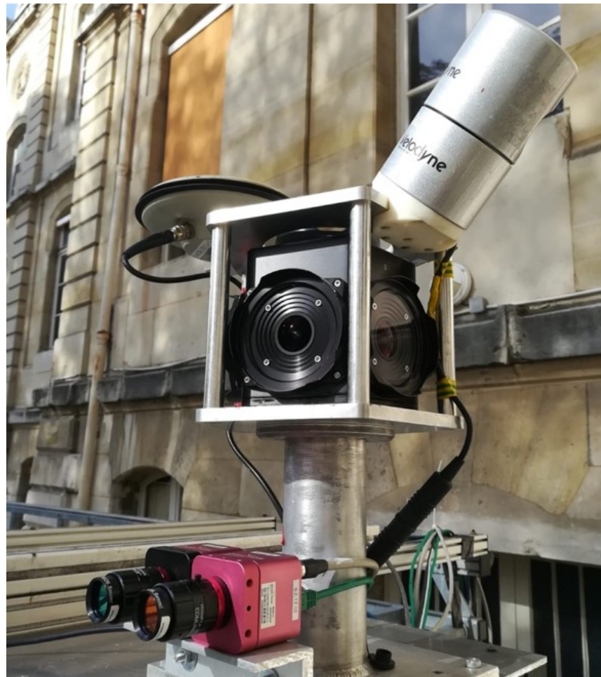
Figure 1. Prototype acquisition system used to create the PC3D dataset in the city of Paris. Sensors: Velodyne HDL32 LiDAR, Ladybug5 360° camera, Photonfocus MV1 16-band VIR and 25-band NIR hyperspectral cameras (hyperspectral data are not available in this dataset; they cannot be used in mobile mapping due to the limited exposure time).
