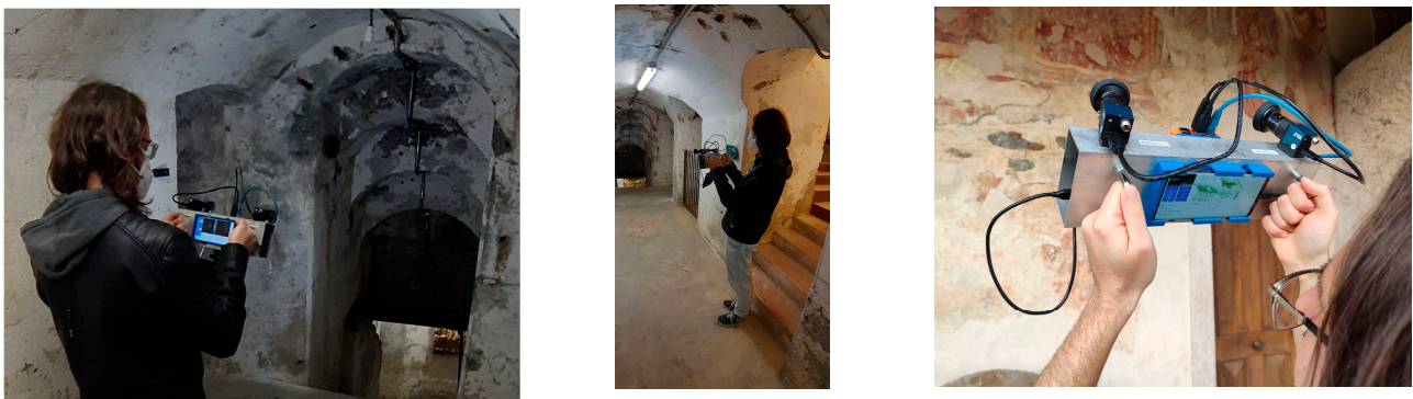
Figure 1. The proposed handheld, low-cost, low-power prototype (named GuPho) based on stereo cameras and V-SLAM method for 3D mapping purposes. It includes a real-time guidance system aimed at enabling optimized and less error prone image acquisitions. It uses industrial global shutter video cameras, a Raspberry Pi 4 and a power bank for an overall weight less than 1.5 kg. When needed, a LED panel can also be mounted in order to illuminate dark environments as shown in the two images on the left.
