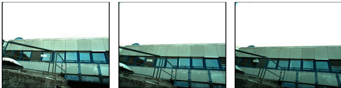
AE algorithm correctly exposed the surveyed object, ignoring the sky overexposure
