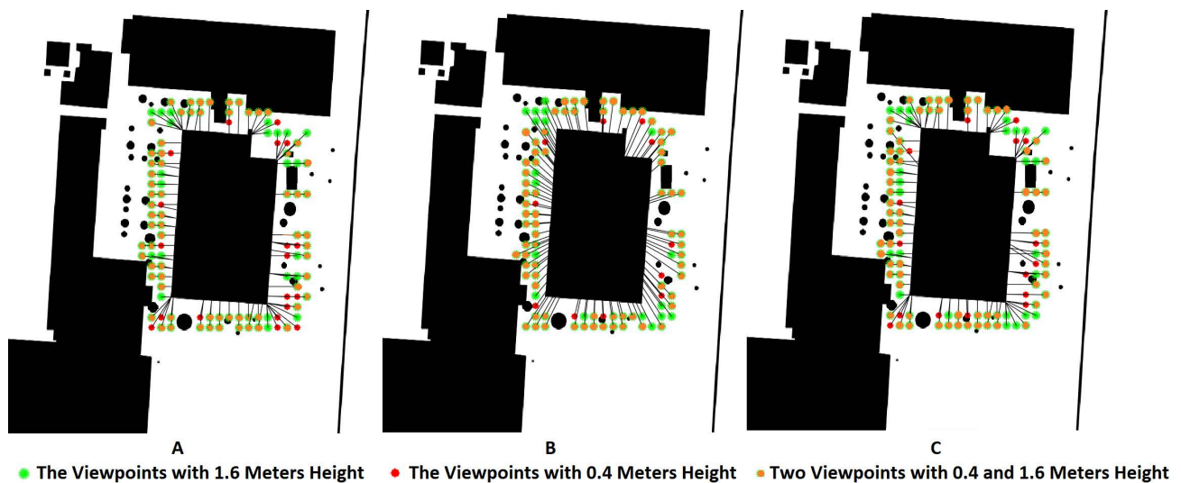
Figure 21. The final vantage viewpoints selected from the candidate viewpoints of the real-world project for the façade pointing (A), centre pointing (B), and hybrid (C) imaging networks.
