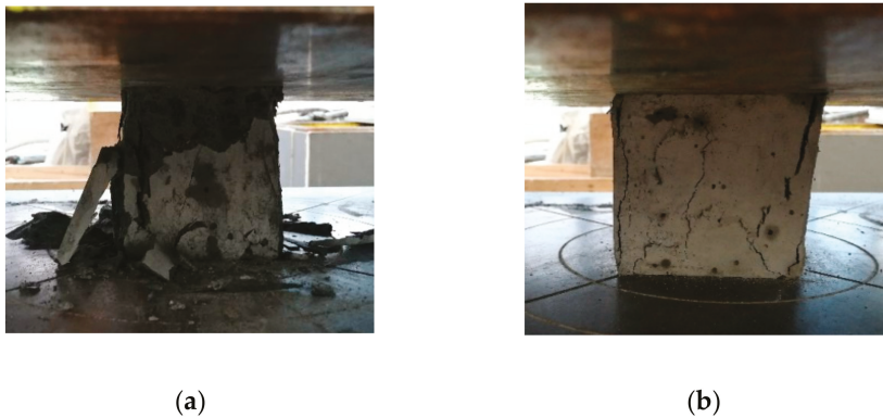
Figure 3. Comparison of compression failure modes of specimens: (a) Reference group; (b) hybrid fiber group.
