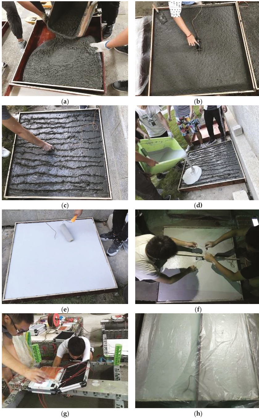
Figure 6. Experimental process: (a) pouring concrete; (b) placing embedded strain sensor; (c) surface processing; (d) pouring GRC material; (e) leveling the GRC surface; (f) placing surface strain sensors; (g) connecting the static strain tester; (h) covering film maintenance.
