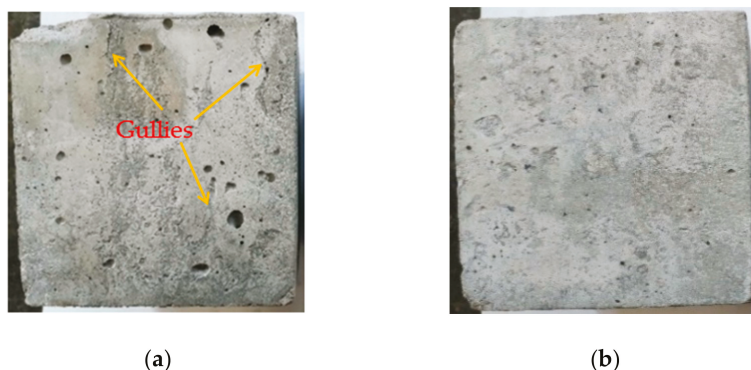
Figure 11. Contrast of morphology of concrete after 100 freeze–thaw cycles: (a) Reference group; (b) hybrid fiber group.
