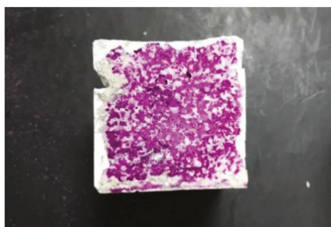
Figure 9. Phenolphthalein test, AC20 specimen (varied w/b ratio and percentage of WPC, 0.4% AEG agent added).
