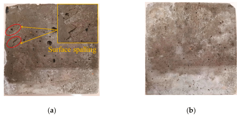
Figure 13. Appearance of specimens after 120 d immersion: (a) Reference group; (b) hybrid fiber group.
