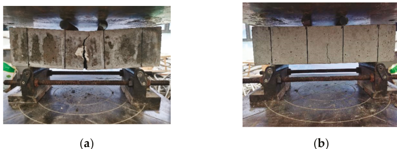
Figure 5. Comparison of flexural failure modes of specimens: (a) Reference group; (b) hybrid fiber group.
