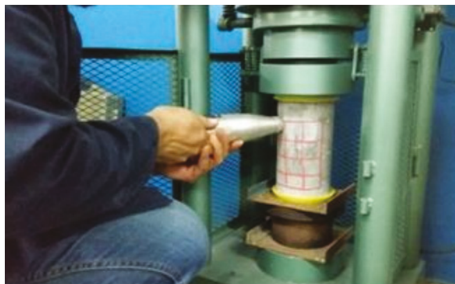
Figure 3. Rebound Number test.
