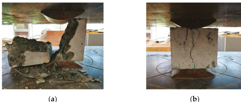
Figure 4. Comparison of splitting failure modes of specimens: (a) Reference group; (b) hybrid fiber group.
