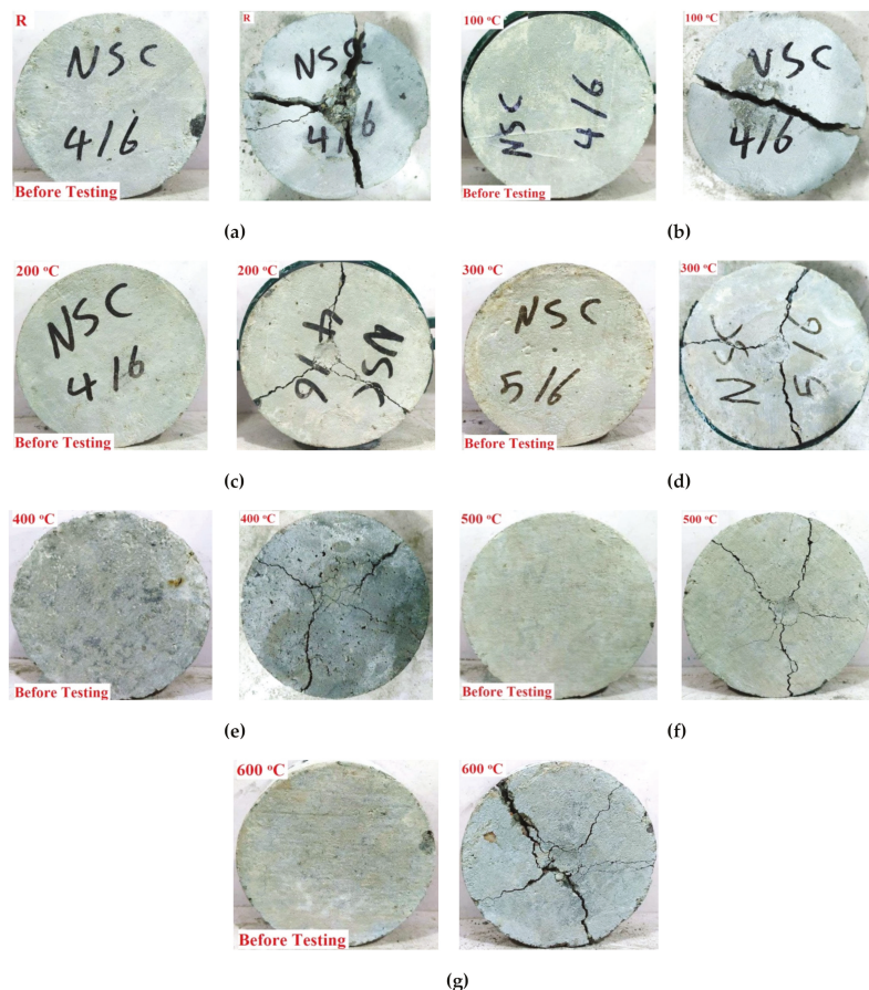
Figure 14. Failure patterns of the impact disc specimens at different temperatures (a) ambient temperature; (b): 100 °C; (c): 200 °C; (d) 300 °C; (e) 400 °C; (f) 500 °C; (g): 600 °C.
