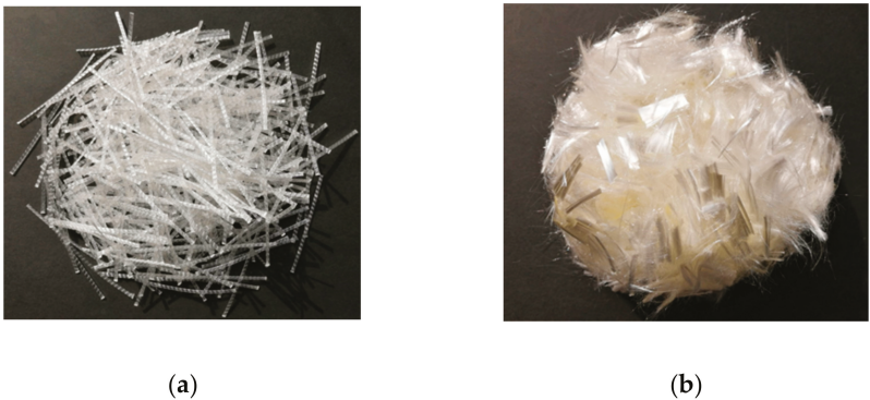
Figure 2. Appearance of fibers: (a) FSTF; (b) PVAF.
