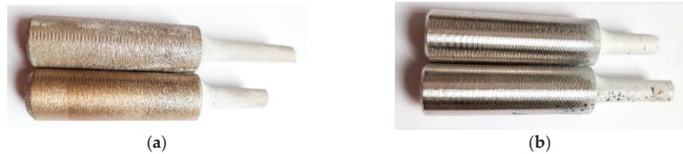
Figure 12. Fractured tensile test specimens: “as printed” (a); machined (b).
