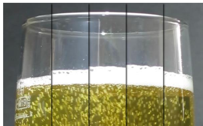
Figure 6. Changes of foam head of sample s02 over time due to the erratic behavior of CO 2 bubbles.
