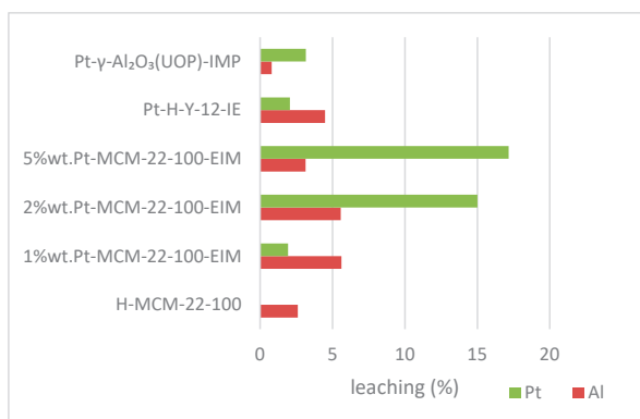
Figure 16. Leaching of aluminum and Platinum (%) in the catalytic ozonation of DCF at 20 °C.
