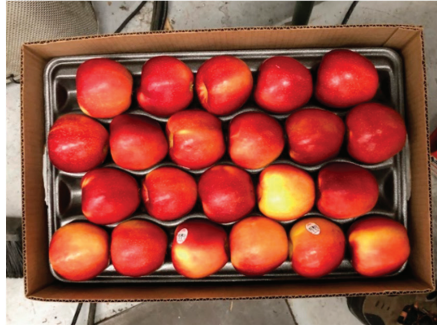
Figure 1. Arrangement of apples in molded pockets prior to testing.
