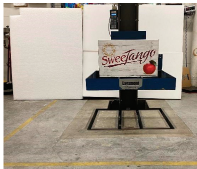
Figure 2. Packaged product on the Lansmont PDT 227.
