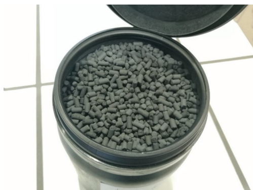
Figure 12. Activated carbon pellets with copper oxide coating.
