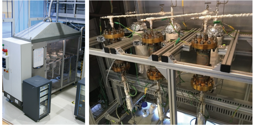
Figure 2. Lab-scale methanation test rig (left); reactors and heat exchangers (right).
