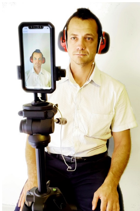
Figure 2. Seated volunteer with Sound Stimulus App, iPhone X, insert earphones, and noise reduction cups.
