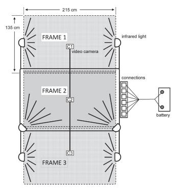
**Figure 2.** Recording system showing the distribution of three video cameras adapted for night vision in the zenith position and six infrared lights connected to a battery. Dimensions of the structure are also showed.
