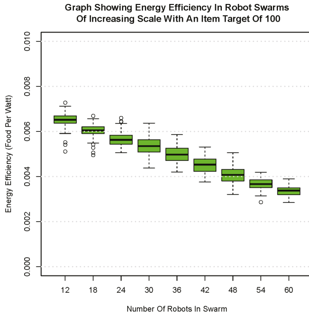
Figure 17. Results for energy efficiency as the number of robots in the swarm increases from 12 to 60.
