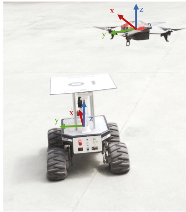
Figure 1. Cooperation between Unmanned Aerial Vehicles (UAVs) and Unmanned Ground Vehicles (UGVs) can greatly benefit Search and Rescue (SaR) tasks where both long-term operation and a wide aerial view are required. The UAV can travel on top of the UGV (possibly recharging its battery) and, when needed, take off, inspect the area, and land again autonomously.
