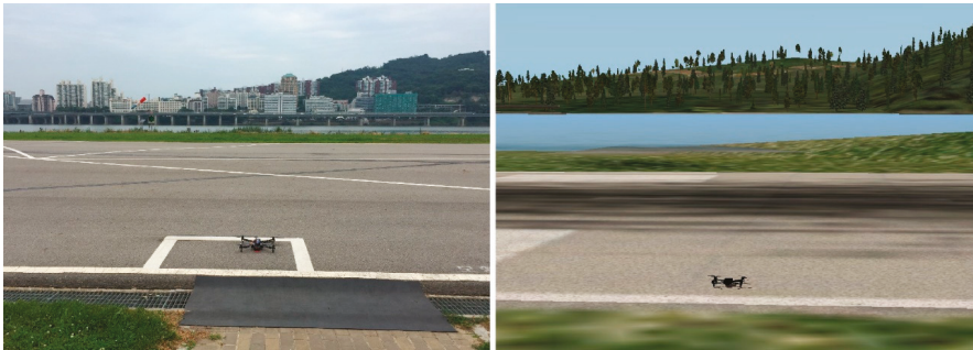
Figure 7. The real quadcopter in the real environment (Hangang Drone Park) (left) and the virtual quadcopter in the X-Plane’s virtual environment (designed Hangang Drone Park) (right).
