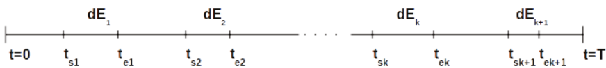
Figure 4. Disconnection events representation. The disconnection events dE_k can appear distributed along the exploration timeline. Its last is variable and depends on the movements realised by the fleet during the exploration. The starting and ending times of each disconnection are represented by the timestamps t_{sk}^i and t_{ek}^i , respectively.
