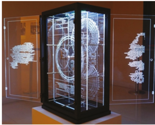
Figure 16. Transparent educational and fully functional model of the Antikythera Mechanism in scale 3:1 (Research team of AUTH-2017).
