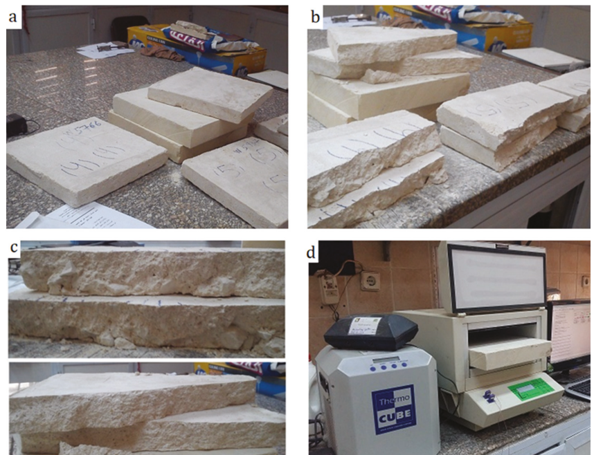
Figure 2. Tested specimens by means of the hot plate for thermal measurements (a) stone, (b) lime-based mortar, and (c) core-infill samples; (d) heat flow meter apparatus.
