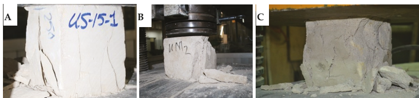
Figure 14. Examples of failure patterns for tested (A) limestone, (B) lime-based mortar and (C) core-infill specimens under uniaxial compression.
