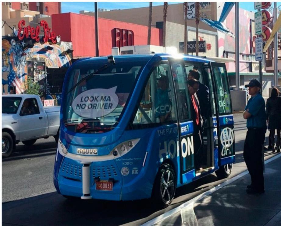
**Figure 4.** Example of an autonomous minibus.
