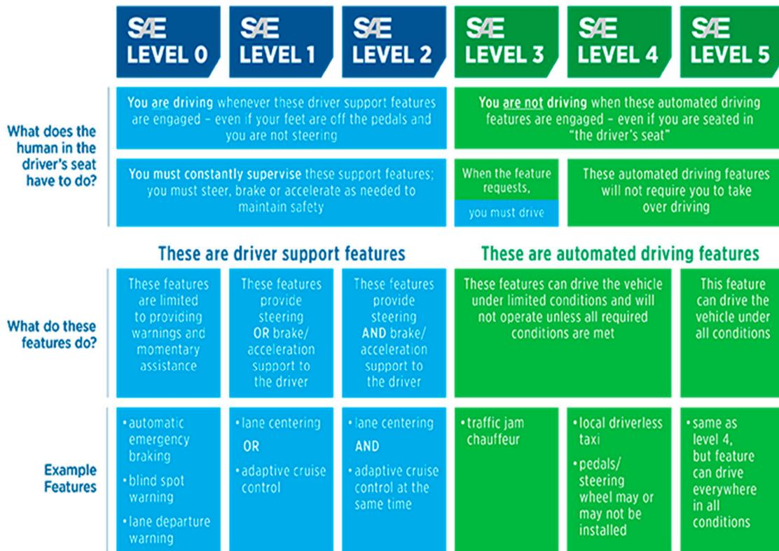
Figure 3. Vehicle automation levels.
