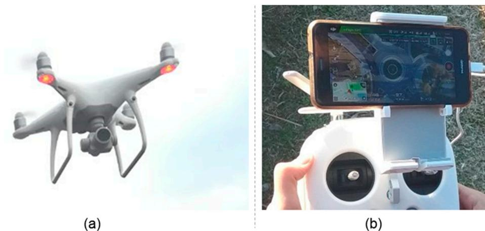
**Figure 6.** (a) The quadcopter UAV and (b) the captured study area as presented on the controller during the survey.
