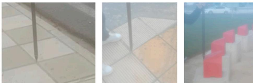
**Figure 4.** Natural ground control points.
