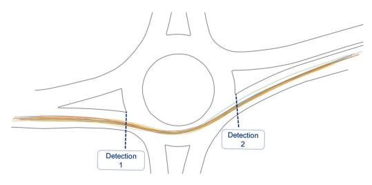
Figure 9. Graphical representation of the vehicle trajectories and the location of coded detectors.
