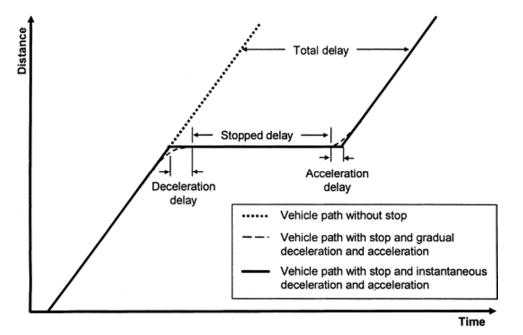
Figure 2. Vehicle delay at intersection.
