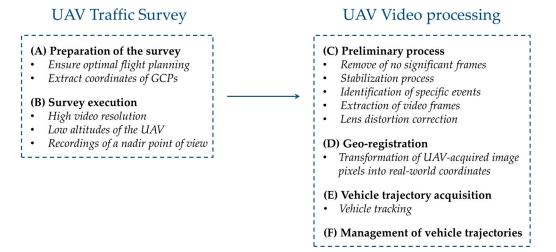
Figure 2. The discrete steps to acquire traffic data using UAVs.
