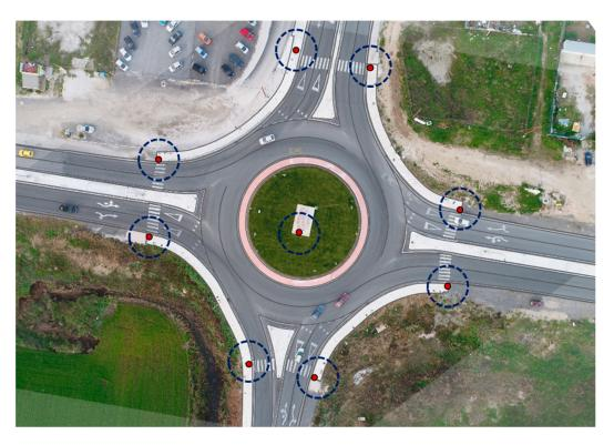
Figure 3. The location of GCPs as distributed homogeneously for the survey.
