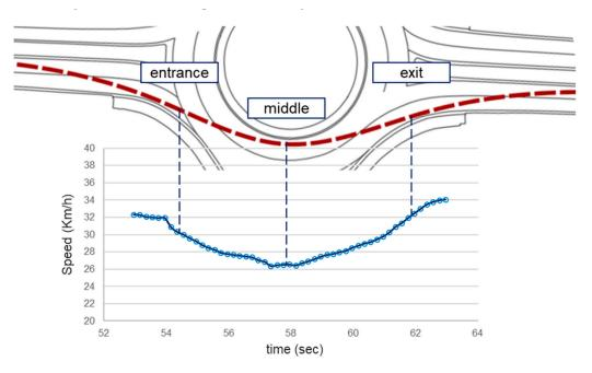
Figure 8. A typical vehicle speed profile has been extracted by processing UAV shots.
