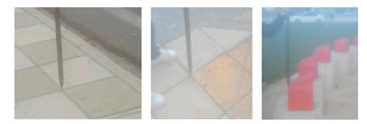
Figure 4. Natural ground control points.
