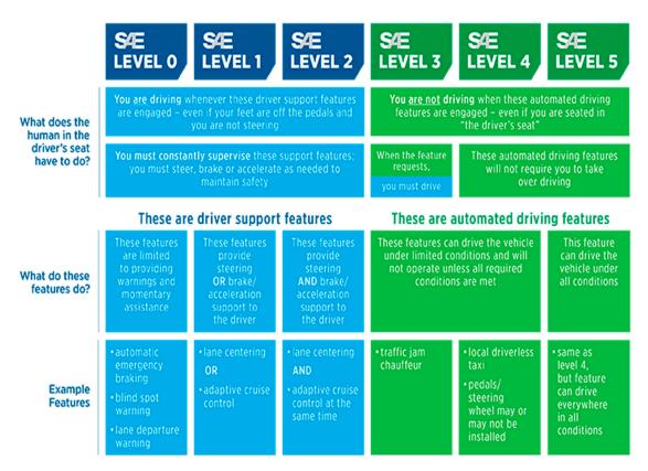
Figure 3. Vehicle automation levels.
