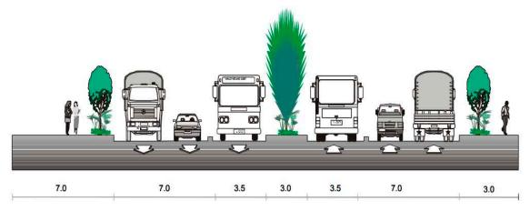
Figure 1. General Bus Rapid Transit (BRT) corridor section, u.m. = meters.
