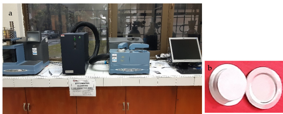
Figure 4. (a) Differential Scanning Calorimeter (DSC) and (b) aluminum sample pan (5 mm).
