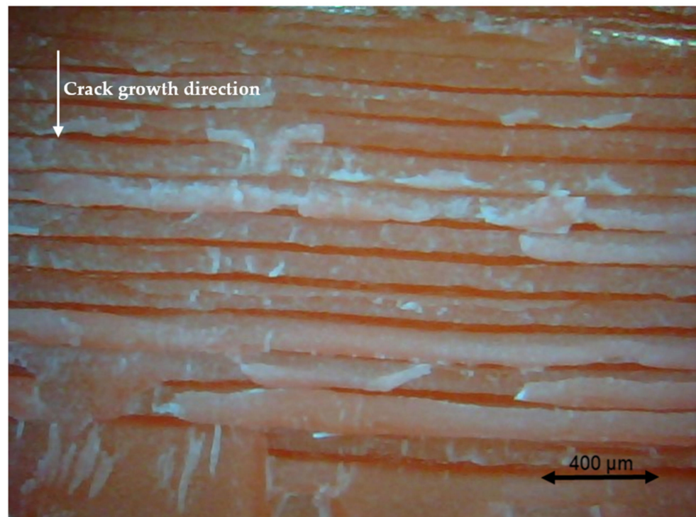
Figure 22. Specimen with a nozzle size of 0.6 mm, Y building orientation, and layer thickness of 0.1 mm.
