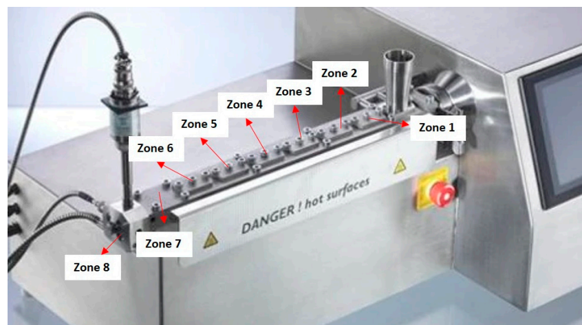
Figure 1. Schematic illustration of the extruder zones.
