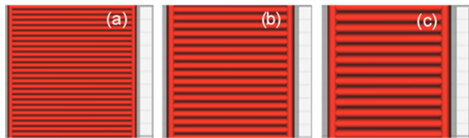
Figure 3. Nozzle size: (a) 0.4 mm; (b) 0.6 mm; (c) 0.8 mm.
