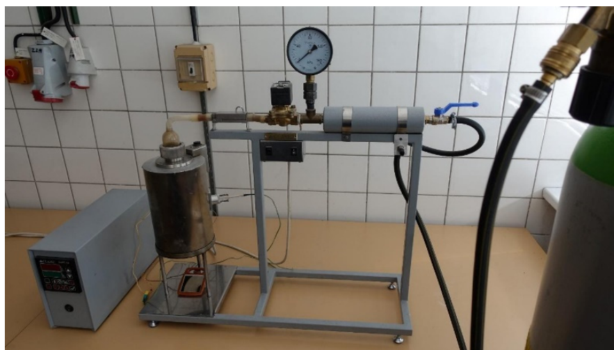
Figure 5. G-G furnace for determination of MIT of dispersed dust.
