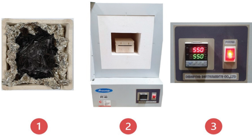
Figure 1. Coupling agent removal processes. 1. Carbon fibers were wrapped with aluminum foil; 2. Placed the carbon fibers with aluminum foil into a Muffle furnace; 3. Set the furnace temperature at 550 °C for 3 h.
