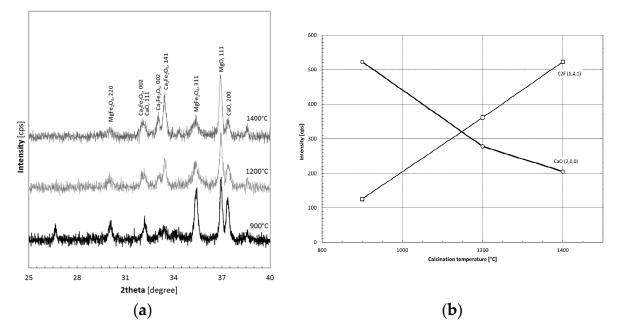
**Figure 7.** Results of phase analysis illustrating the solid-phase chemical reactions occurring during heating the raw magnesite: (a) identified products at various temperatures, (b) conversion of free lime to dicalcium ferrite ( $2CaO \cdot Fe_2O_3$ ).
