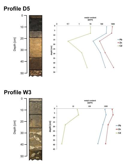
**Figure 3.** Characteristic examples of studied soil profiles in elevated- (profile D5) and buried (profile W3) ore-bearing dolomitic areas (photographs: T. Hulok).
