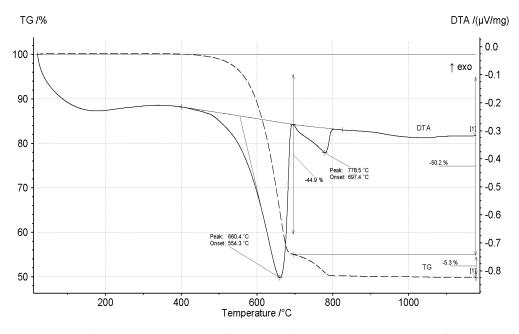
**Figure 2.** Results of thermal analysis illustrating the thermal decomposition of magnesite and dolomite during heating the raw magnesite.
