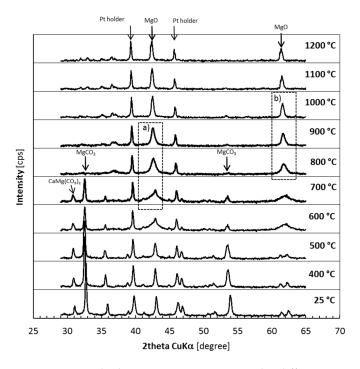
**Figure 3.** In situ high-temperature X-ray powder diffraction sequence illustrating the changes in phase composition and crystallinity during heating the raw magnesite. (Magnesite and dolomite reflections gradually disappear above 700 °C (frame "a"), and the new phase of periclase is created (frame "b").).
