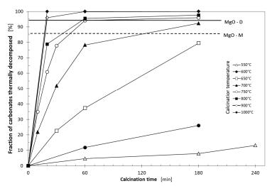
**Figure 4.** Influence of temperature and time on fraction of carbonates decomposed during heating the raw magnesite.
