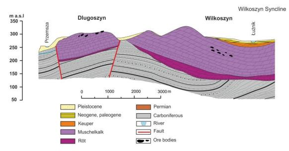
**Figure 1.** Schematic geological cross-section of the study area showing location of ore bodies, without Quaternary sediments (after [54]).
