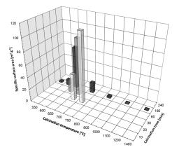
**Figure 9.** Influence of calcination temperature and time on specific surface area during heating the raw magnesite.
