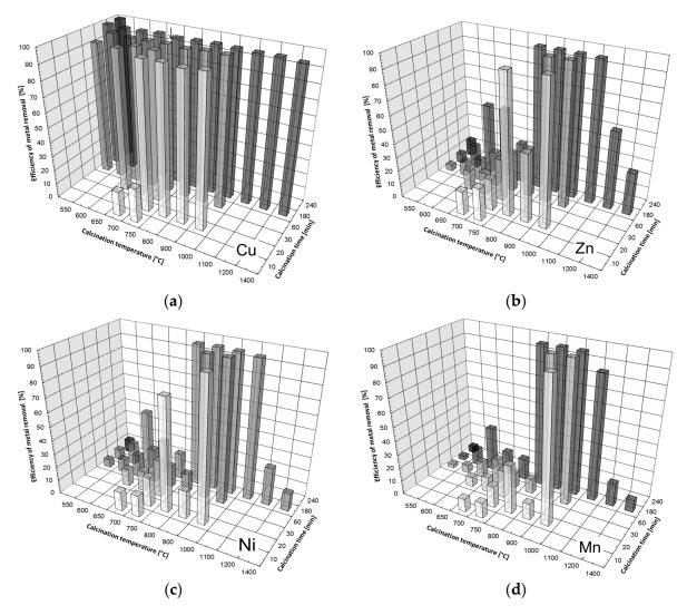
**Figure 5.** Influence of calcination temperature and time on the efficiency of monitored metal removal from the model solution by addition of the CCM tested: (a)  $Cu^{2+}$ , (b)  $Zn^{2+}$ , (c)  $Ni^{2+}$ , and (d)  $Mn^{2+}$  using a liquid-to-solid ratio l:s = 200:1.
