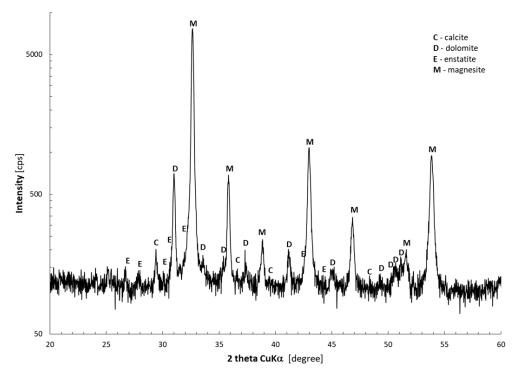
Figure 1. XRD analysis of the raw magnesite used for the experiments.
