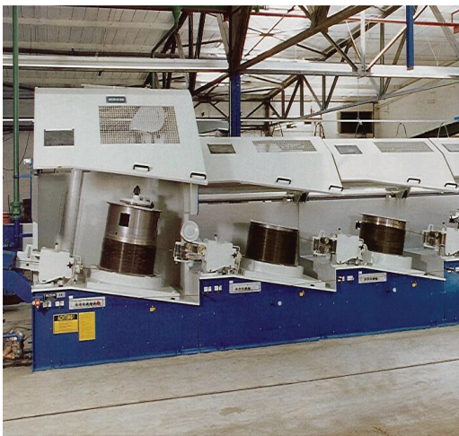
Figure 1. Manufacture of prestressing steel wires by progressive cold drawing of a previously hot-rolled pearlitic steel bar: two views of a real manufacturing chain by progressive (multi-step) cold drawing.
