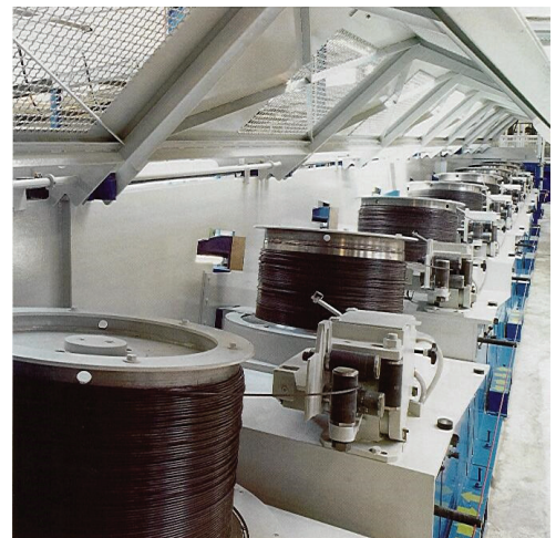
Figure 1. Manufacture of prestressing steel wires by progressive cold drawing of a previously hot-rolled pearlitic steel bar: two views of a real manufacturing chain by progressive (multi-step) cold drawing.
