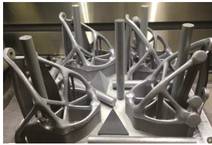
Figure 9. Build plate with 4star tracker camera bracket components.
