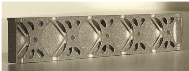
Figure 15. As-printed image of the sectioned Edge insert.
