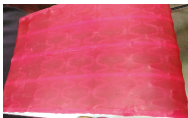
Figure 15. Pre-tensioned latex skin covering a wing partition.
