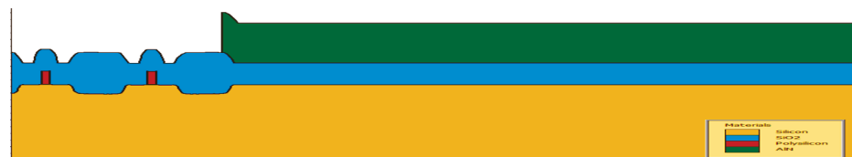
Figure 2. AlN piezoelectric layer deposition.
