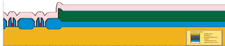
Figure 3. Metal layers deposition.
