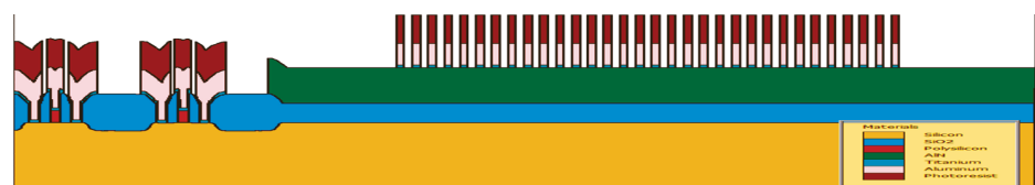
Figure 5. Titanium and aluminum etch.
