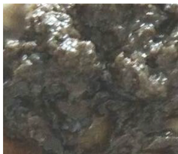
Figure 3. Intercepted oil pollution on the surface of the filter layer.
