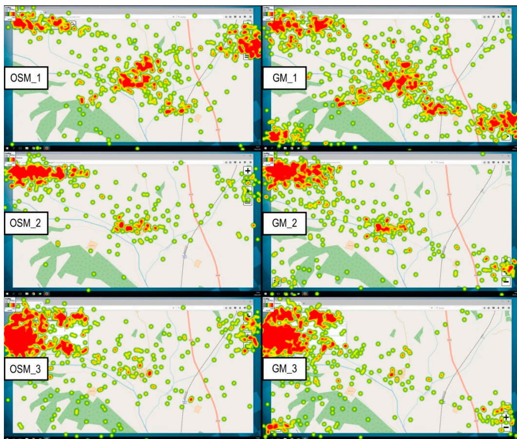
Figure 7. Six heatmaps presenting the spatial distribution of fixations in each task on both GUIs. OSM (from 1 to 3) stands for the OpenStreetMap-based GUI, and GM (from 1 to 3) stands for the Google Map-based GUI.
