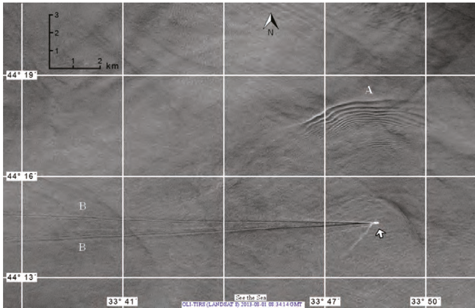
Figure 12. Different types of IWs propagating near the south coast of Crimea: (A) natural IW; and (B) IW generated by a moving ship, arrow points to the ship; Landsat-8 OLI (panchromatic band, resolution 15 m), 1 August 2013.
