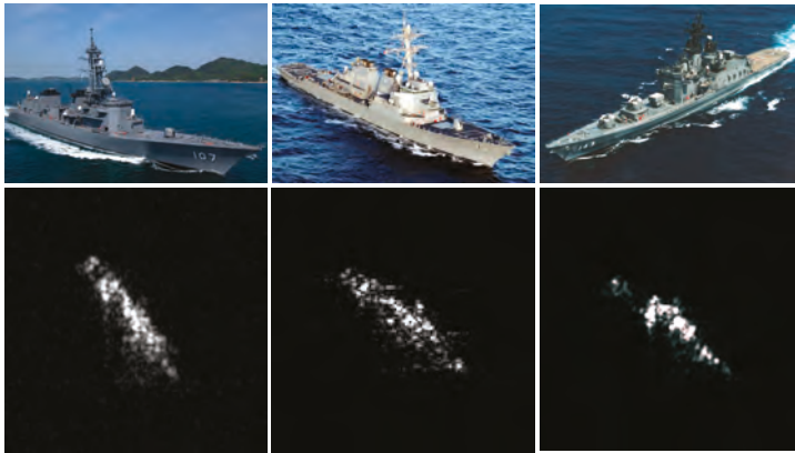
Figure 1. The optical and synthetic aperture radar (SAR) images of different types of ships.
