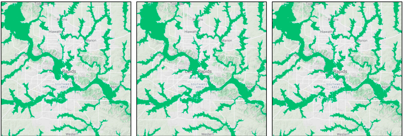
Figure 6. Maps generated for Cedar Rapids, Iowa with HAND model using 10 m, 25 m, and 50 m (left to right).
