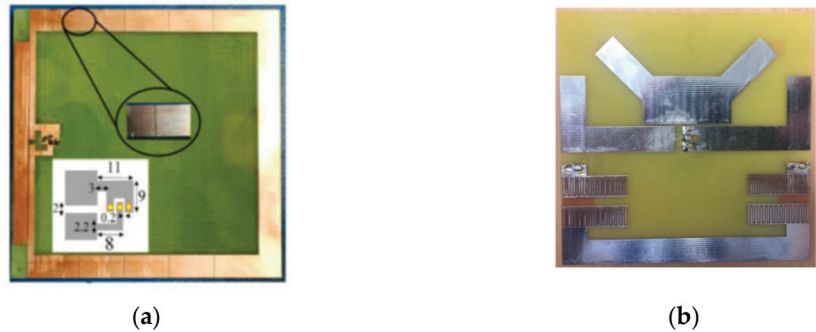
Figure 14. MNG loaded antennas: (a) MNG loaded loop antenna (reproduced with permission from [60], Copyright 2016 IEEE); (b) MNG loaded reflector Yagi-antenna. Reproduced with permission from [75]. Copyright 2017 IEEE.
