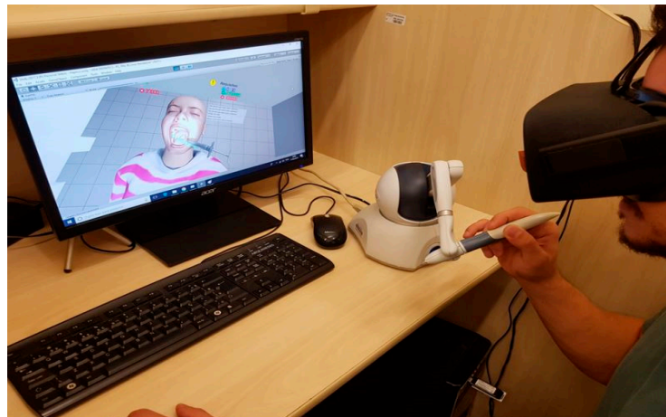
Figure 3. A user conducting a dental anaesthetic procedure using a haptic device [31], reproduced with permission from Nunes, F.L.S.
