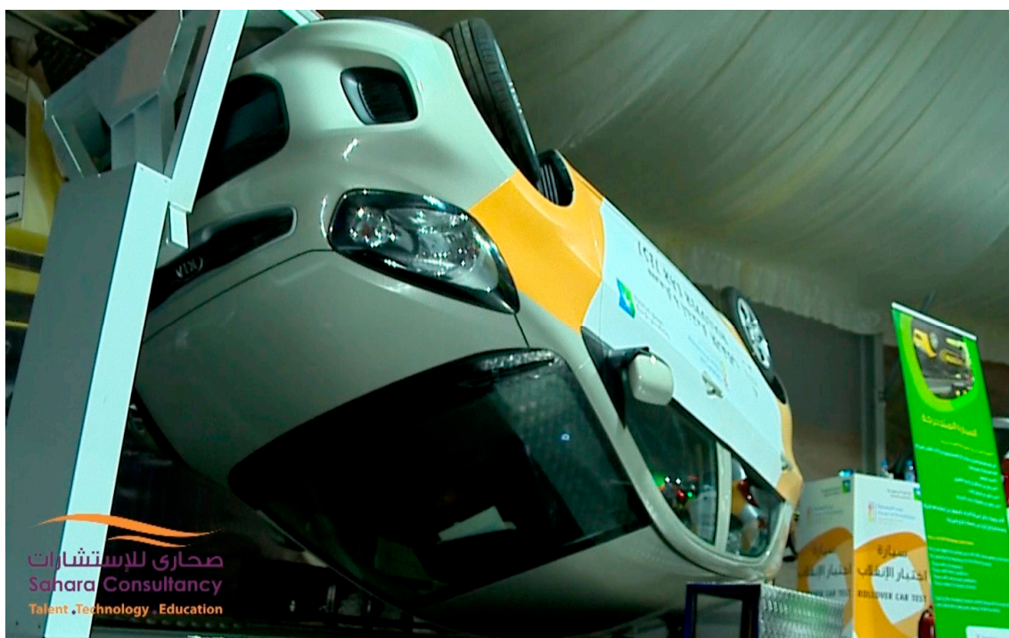
Figure 3. The rollover simulator with the car turned upside down (180° turn).
